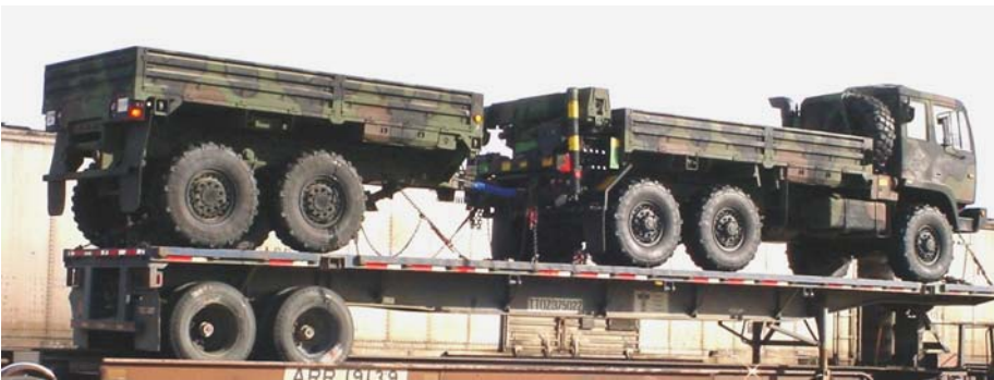
Medium truck and trailer. Overall good securement. Needs strap on tongue of trailer.
