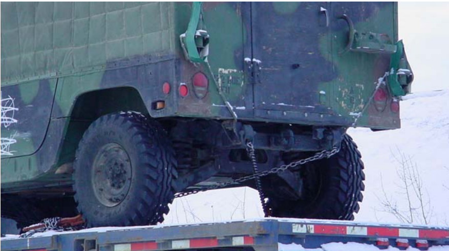
Good example of cross chaining to the center.
