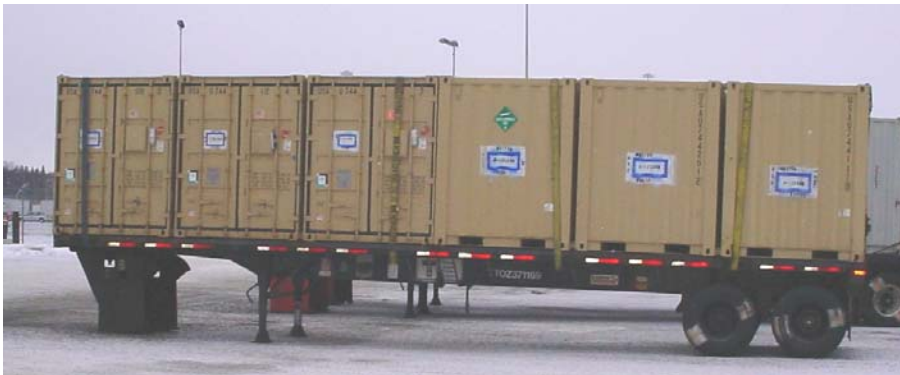
Two Tri-Con packages loaded on 40' trailer.
