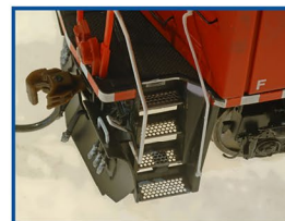
Etched, see-through walkway steps
