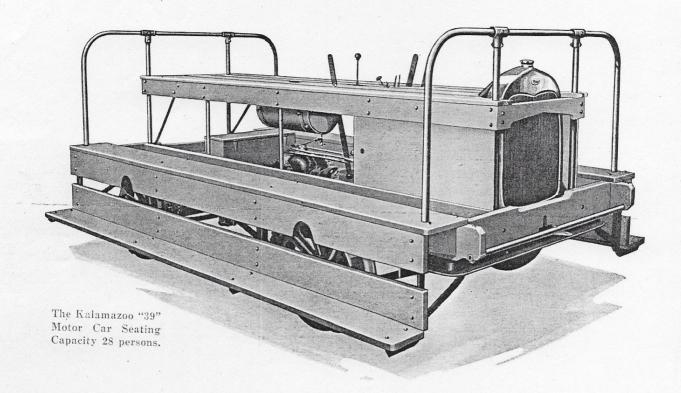
HE Kalamazoo "38" and "39" Motor Cars are equipped with the standard Model "A" Ford Engine which develops 39 brake H.P. at 2200 R.P.M. It is exceptionally economical on gasoline and oil. The standard Ford starter, generator, battery and ignition are regular equipment. Lights furnished if desired at slight additional charge.
