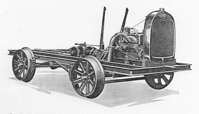
Car frame is constructed of 3 channel steel riveted and welded at all joints and securely trussed.
