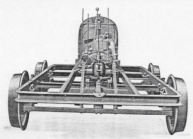
Note the rugged Kalamazoo reverse transmission driving from both sides through heavy duty roller chains to the axle. This method of drive equalizes the strain on the transmission which assures longer life of the transmission and chains.
